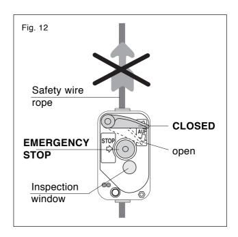
b) Open the BSO secondary brake again by pressing the lever down and jerk the safety rope – the blocstop® must close automatically: if not, replace and send it to the supplier
