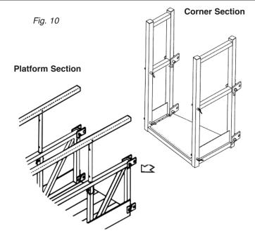
Use H-bracket Connectors with Rigid Platform Sections (Note "U" Frames can be substituted for "H" Brackets if needed for rigid platforms.)
