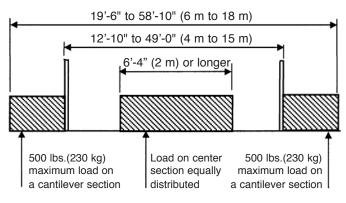
Note: Only use 9'-8" (3m) sections on both ends of any platform using Intermediate Stirrups. Joints should not be beyond the stirrup.
