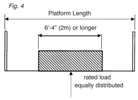
Note: The rated load should be located in the center of the platform and distributed over a length of at least 6'-4" (2m). (see Fig. 4 above)
