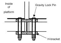
H-Connector/Gravity Lock Pin Connection Details
