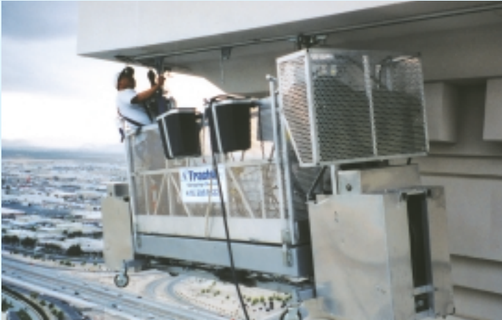
TRACMOD suspended from monorail track with suspension trolleys.
