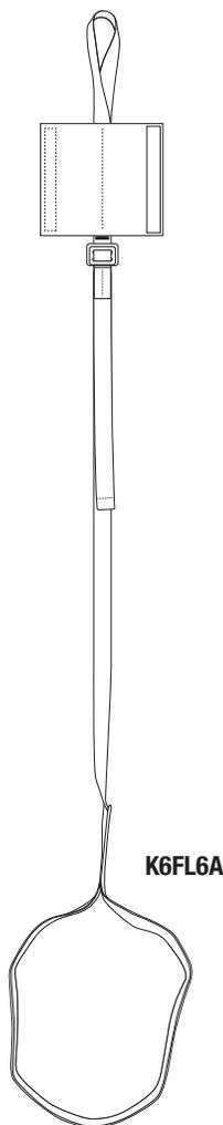
The post fall suspension loop is a specialized fall arrest rescue accessory designed for use within a post fall situation. Primarily designed as a tool to alleviate circulatory restriction created from being under suspension within a fall arrest harness, the suspension loop allows the user to transfer the pressure that the harness creates upon the femoral artery onto the suspension loop, alleviating pain and discomfort.
