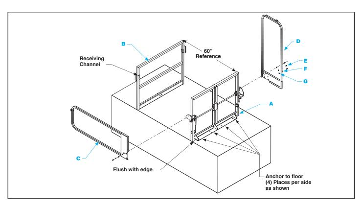
Safety Note: There must be OSHA-approved fall protection devices in use during the installation of this product! Assemble the unit away from the edge of the mezzanine. After assembly is complete, move the MZ Clear Height Safety Gate to the edge as shown and anchor to the floor.
