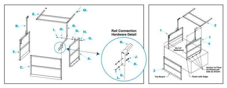
Safety Note: There must be OSHA-approved fall protection devices in use during the installation of this product! Assemble the unit away from the edge of the mezzanine. After assembly is complete, move the MZ-Pivot Gate to the edge as shown and anchor to the floor.
